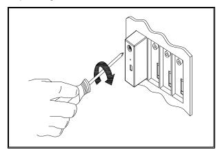
Step 4: Connect to CAN Bus network. The CAN Bus transmitting device and the KCU-04 connection must follow CAN-High connect to CAN-H, CAN-Low connect to CAN-L and shielded line connect to Shield.
