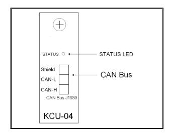
It is strongly suggested to use shielded dual-core braided harness for CAN Bus wiring connection with shielded grounding harness on one side.
